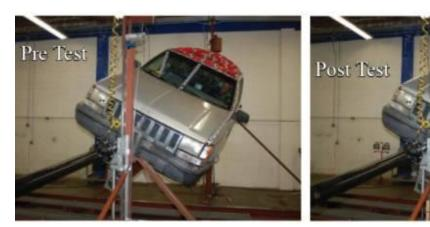
Figure 6. HALO<sup>TM</sup> Prototype 2; No noticeable deformation to the roof structure
