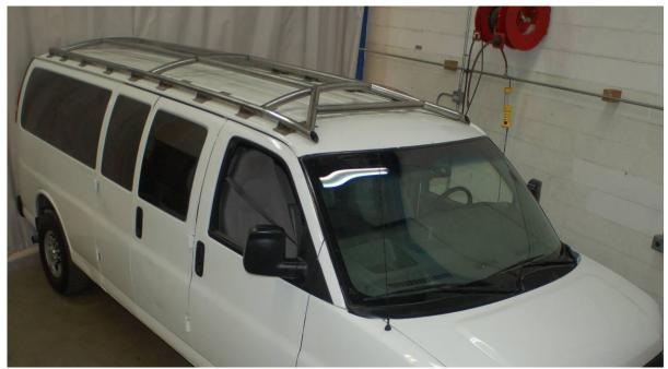
Figure 18. 12 to 15 Passenger van with HALO<sup>TM</sup> rollover load distribution device.
