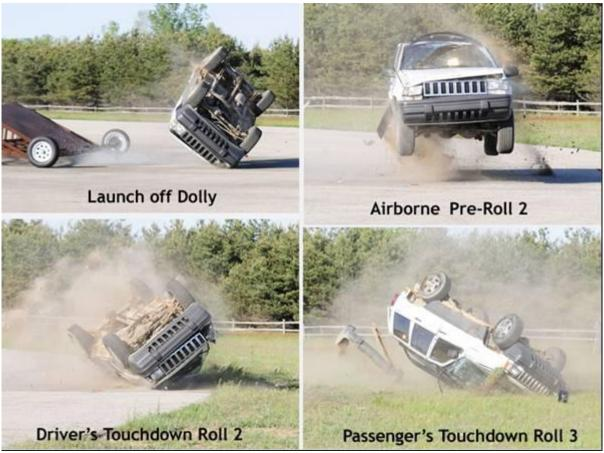
Figure 10. HALO<sup>TM</sup> Prototype 4 during a FMVSS 208 dolly rollover test
