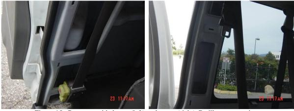
Figure 15. Passenger-side lower (left) and upper (right) C-pillar open sections
