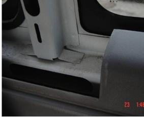
Figure 13. Non-structural pillars
