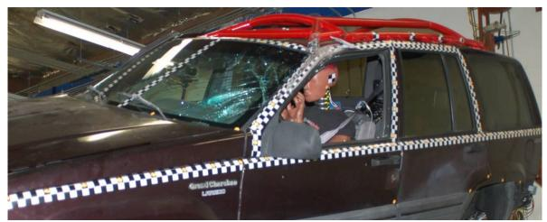
Figure 9c. HALO<sup>TM</sup> Prototype 4 Roll 2 post-test photograph
