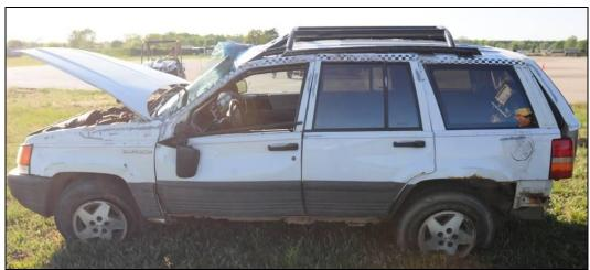
Figure 11. Prototype 4 HALO<sup>TM</sup> after a 3 roll dolly rollover test
