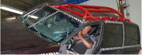
Figure 9d. HALO<sup>TM</sup> Prototype 4 Roll 3 post-test photograph
