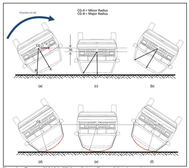
Figure 4. Top row: Vehicle's CG drops during rollover and then rises again;
