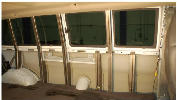
Figure 17. Passenger van internal retrofit strengthening system
