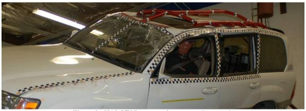
Figure 8. HALO<sup>TM</sup> Prototype 3 post-test photograph
